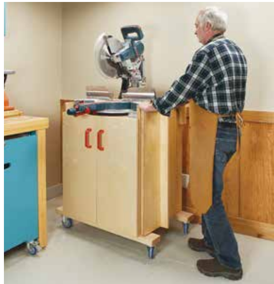
▲ With the wings folded down, the swivel casters allow you to easily maneuver the miter saw station into a corner of your shop, until the next time you need it.
