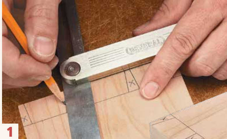
▲ Layout Marks. With a bevel gauge set to the proper dovetail angle, mark the tail locations on a test piece.
