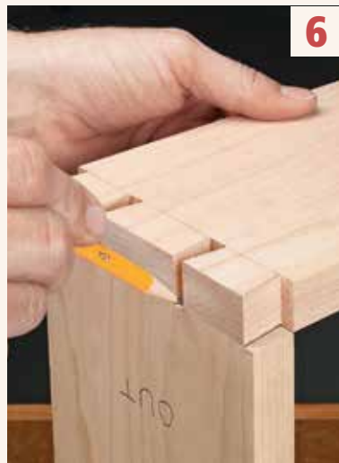
▲ Locate the Pins. Use the completed tail workpiece with the original layout to locate the pins on the mating workpiece.
