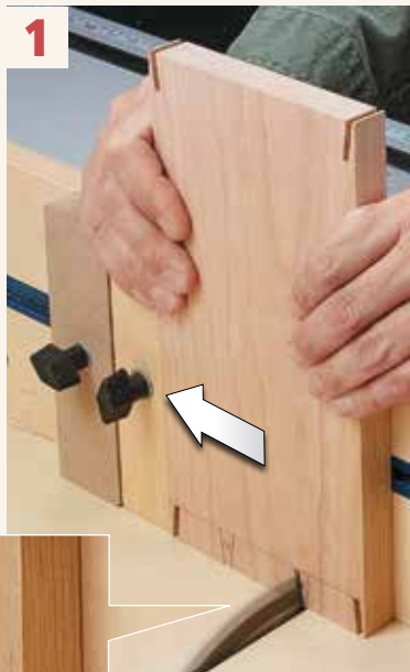
▲ Second Cuts. At this point, the spacer accurately controls the position of the workpiece for the next cut.
