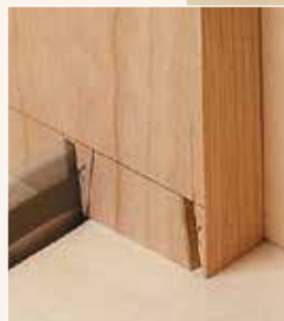
▲ Second Cuts. At this point, the spacer accurately controls the position of the workpiece for the next cut.
