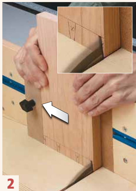
▲ Set the Stop Block. After aligning the layout mark with the blade, lock the stop block into position and make the first cut.
