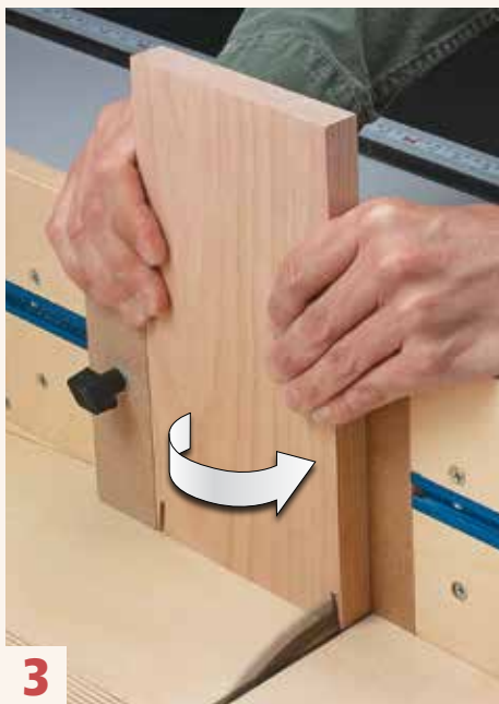
▲ Cut and Turn. Rotate the workpiece to make a matching cut on the opposite side. This technique ensures uniform spacing.
