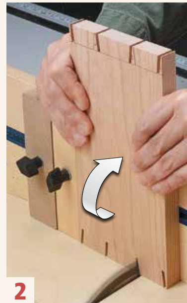
▲ Both Ends. As before, flip the workpiece over and repeat the cuts on both ends.
