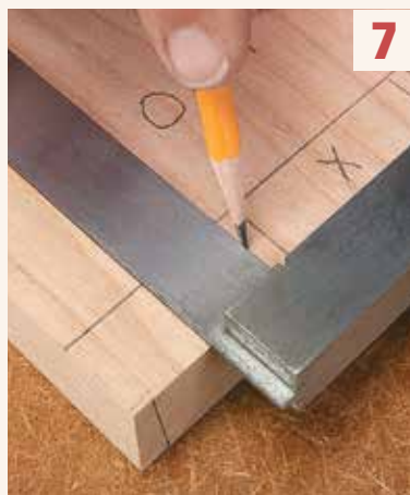
▲ Transfer. Transfer the layout marks down the front face of one workpiece. Finally, mark the outside face of all the pin workpieces.
