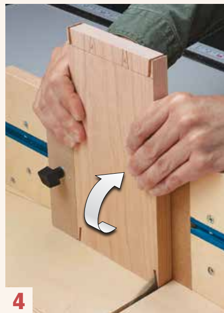
▲ Both Ends. Flipping the workpiece end-over-end allows you to make identical cuts on the opposite end.
